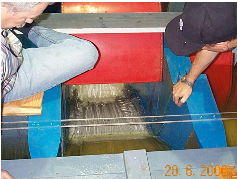
Picture 16. "Rough" RSW alt 7 w/o ramp. Double ogee and "rooster tails".
