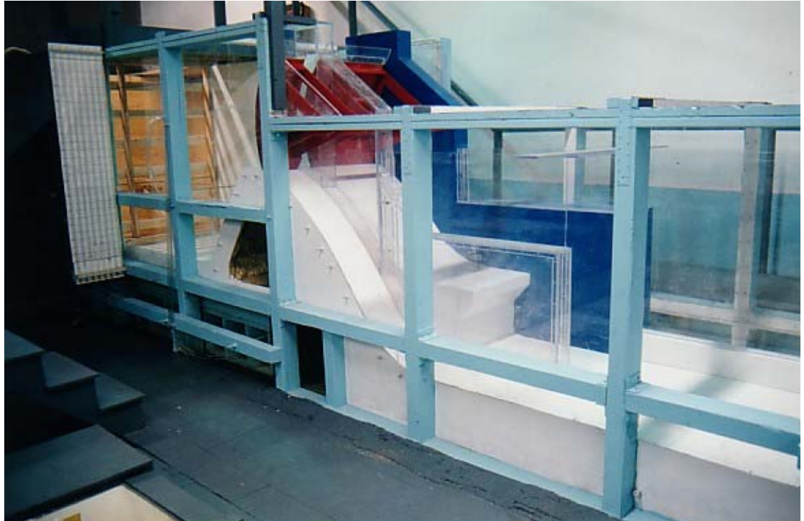
1) View of the John Day Bay 20 50 ft deflector geometry with the existing spillway crest geometry. (R22-04)
