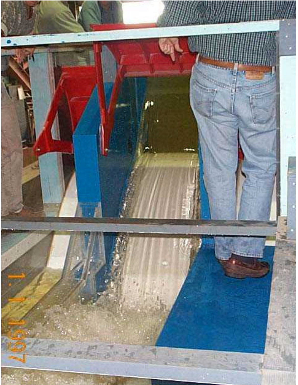
Photograph 2. RSW Alt 2, Standing Waves & Roostertails Down Spillway Face
