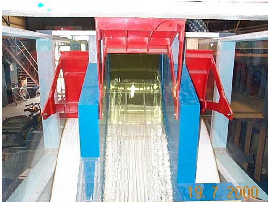
Photograph 12. RSW 5, Flow Down Spillway Face
