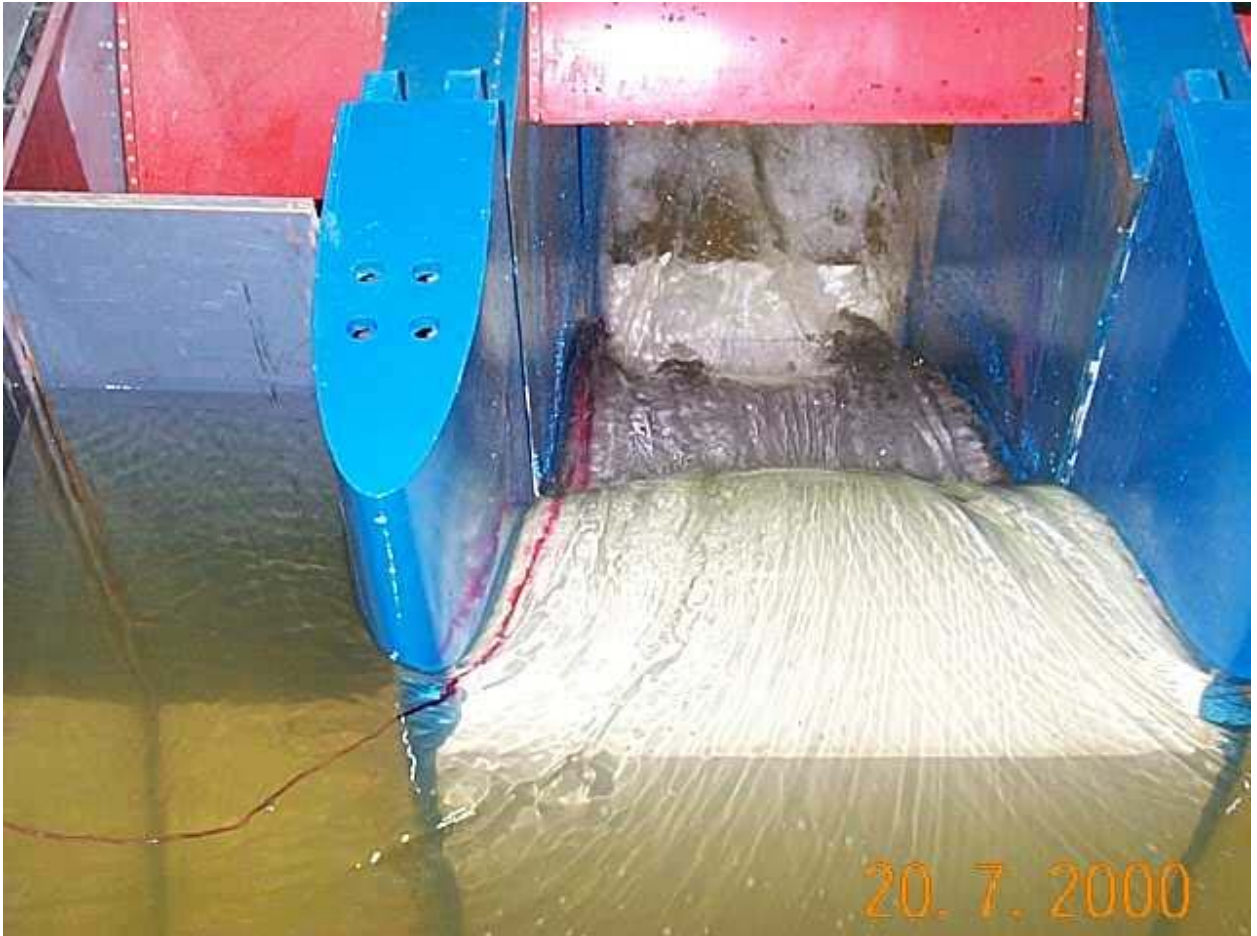
1) Alternative 2: View of the water surface patterns looking from upstream of the RSW and existing spillway crest.
