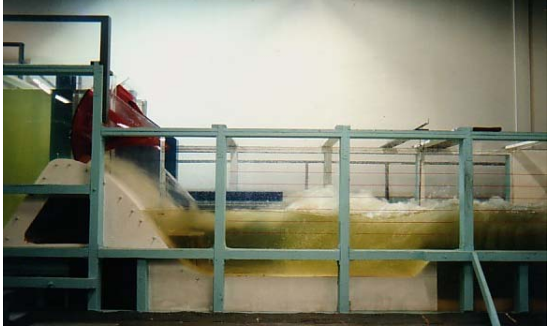
1) 30 ft Deflector Discharge 40,000 cfs/bay (800,000 cfs project discharge); Forebay Water Surface Elevation 268.0 ft Tailwater Elevation 173.0 ft. (R2A-23)
