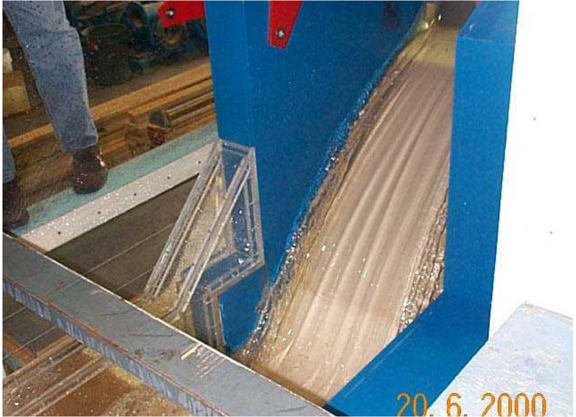
1) Alternative 5: View of the water surface patterns looking from downstream over the stilling basin. Note the relatively smooth water surface when compared to the flow patterns over Alternatives 2 and 4.
