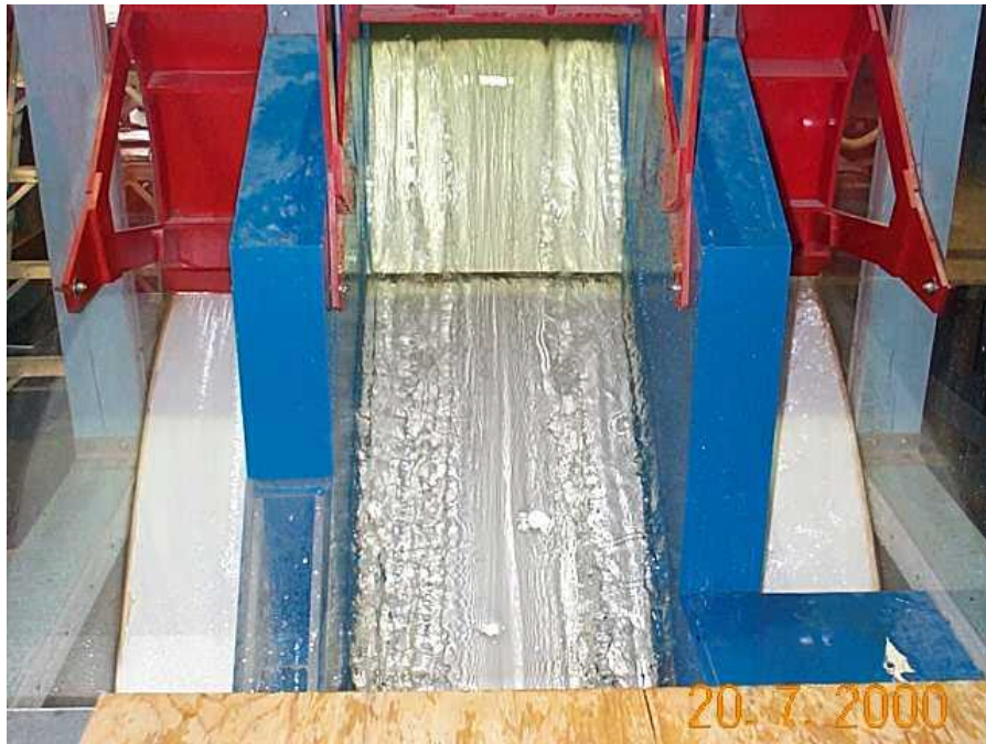
Photograph 9. RSW Alt 4, Standing Waves Both Up and Downstream of Step
