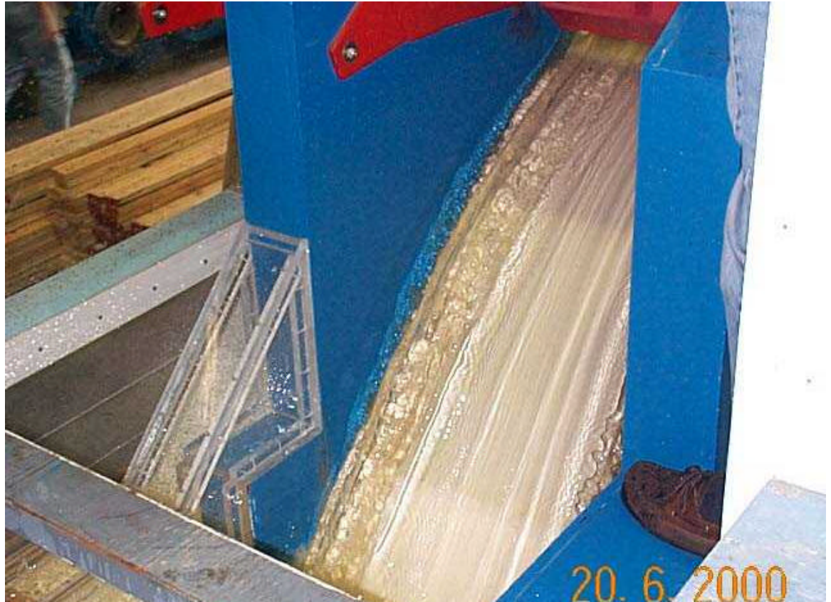
Photograph 16. RSW 7 (Simplified). Flow Conditions With Spillway Gate Control
