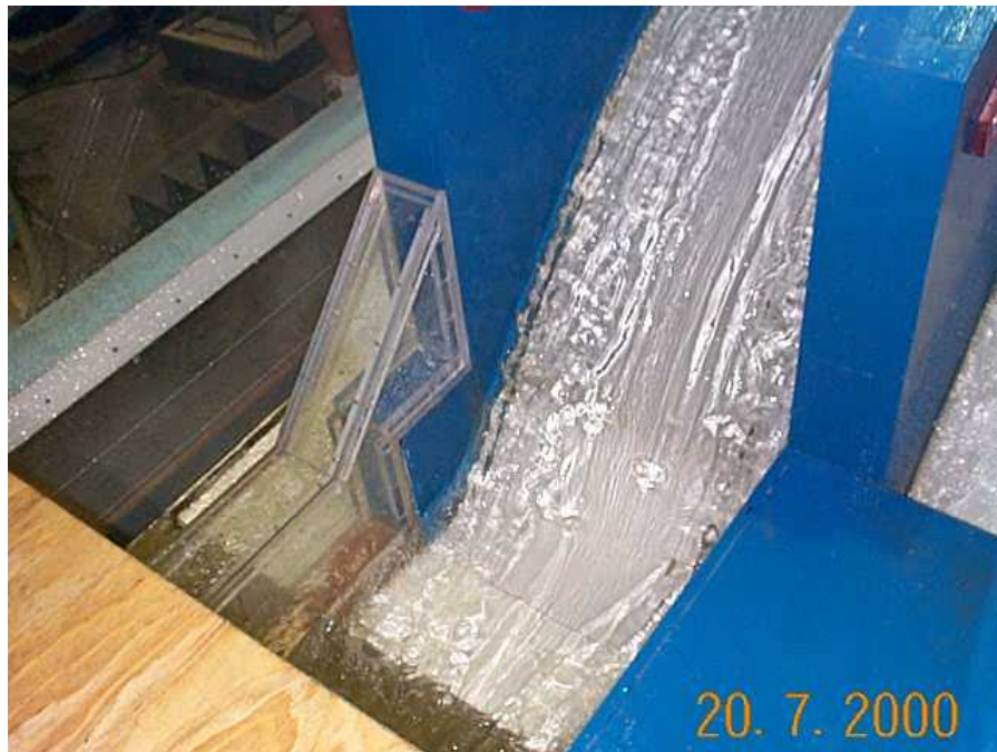
Photograph 9. RSW Alt 4, Standing Waves Both Up and Downstream of Step
