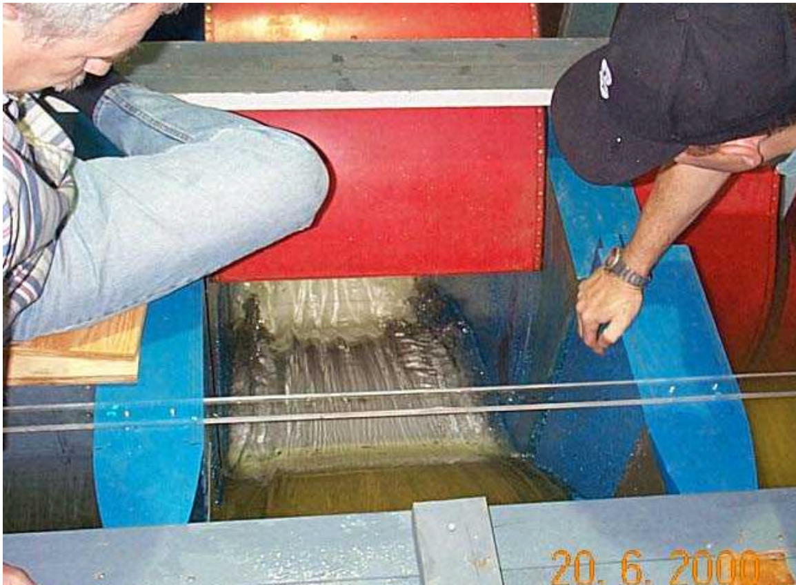
Photograph 14. RSW 7 (Simplified). Standing Waves on Spillway Face
