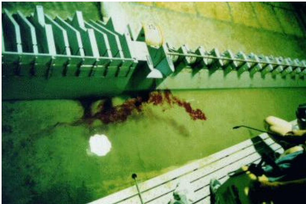
Photograph 6. RSW Alt 2, Approach Conditions, 15.3 kcfs, Total Q 350kcfs, 30% Total Flow Over Spillway (91.2 kcfs)
