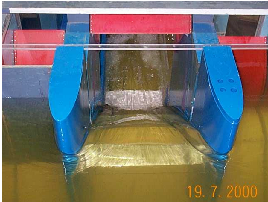
Photograph 11. RSW Alt 5, Drawdown Around Piers & Flow Over Crest
