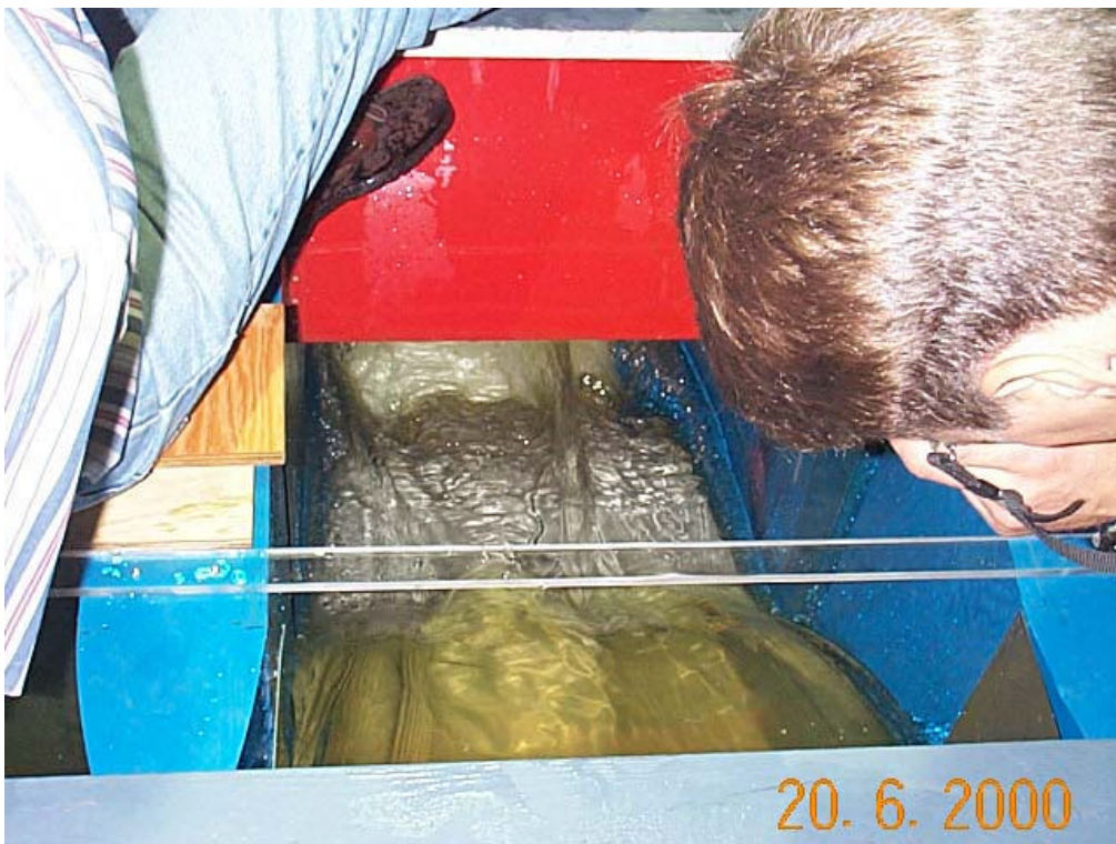
Picture 12. "Rough" RSW 7. Double ogee (inflection) and "rooster tails".
