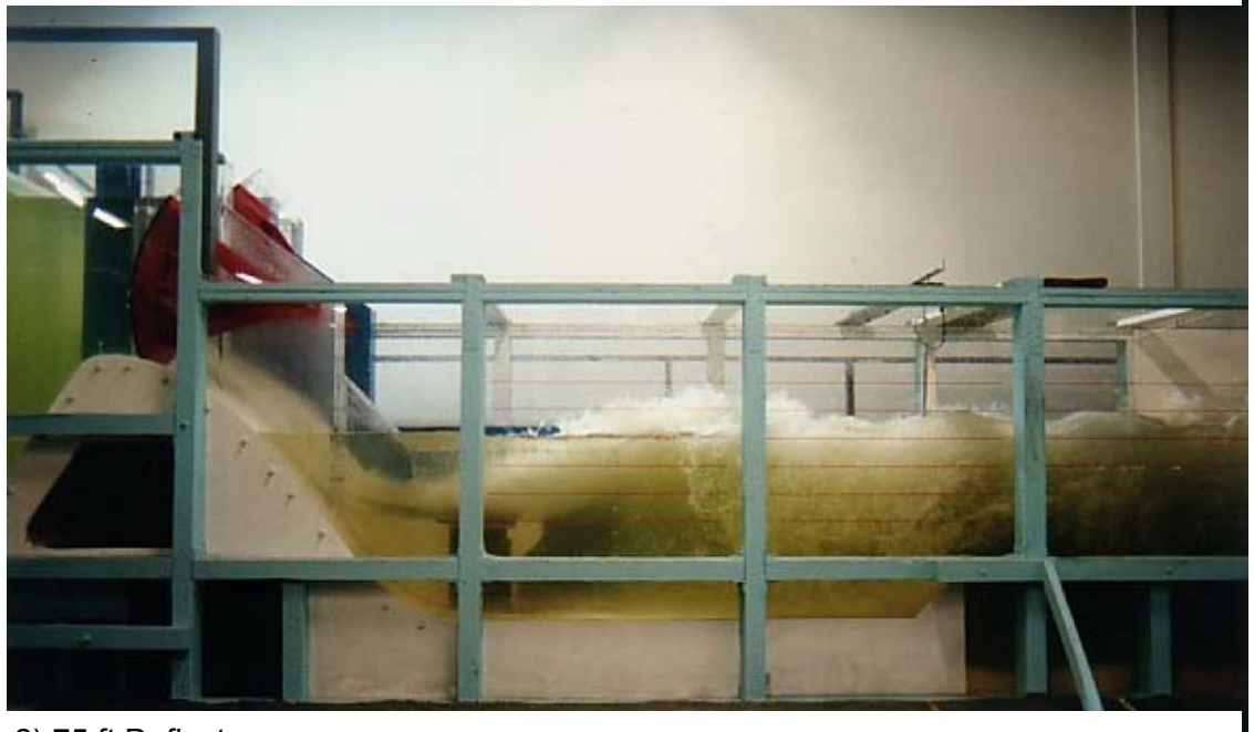
2) 75 ft Deflector Discharge 40,000 cfs/bay (800,000 cfs project discharge) Forebay Water Surface Elevation 268.0 ft Tailwater Elevation 186.5 ft. (R2A-11)
