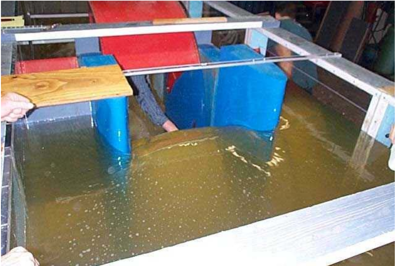
1) Alternative 2: View looking downstream at the water surface drawdown around the pier additions.
