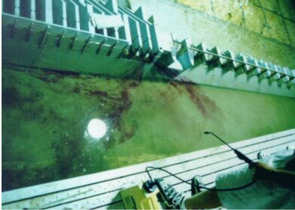
Photograph 7. Skeleton Bay Collector, Approach Conditions, 18.9 kcfs, Total Q 250kcfs, 30% Total Flow Over Spillway (56 kcfs)
