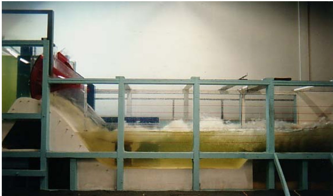
2) 75 ft Deflector Discharge 40,000 cfs/bay (800,000 cfs project discharge); Forebay Water Surface Elevation 268.0 ft Tailwater Elevation 173.0 ft. (R2A-23)
