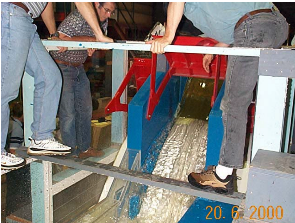
Picture 14. "Rough" RSW alt 7 w/o ramp. "Rooster tails".
