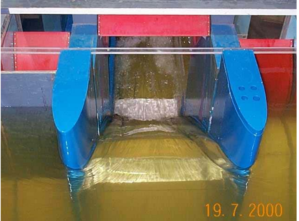
1) Alternative 5: View of the water surface patterns looking from upstream of the RSW and existing spillway crest.
