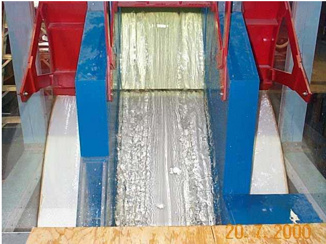
1) Alternative 4: View of the water surface patterns looking from downstream over the stilling basin. Note the 2 ft step at the transition between the RSW and the existing spillway crest.
