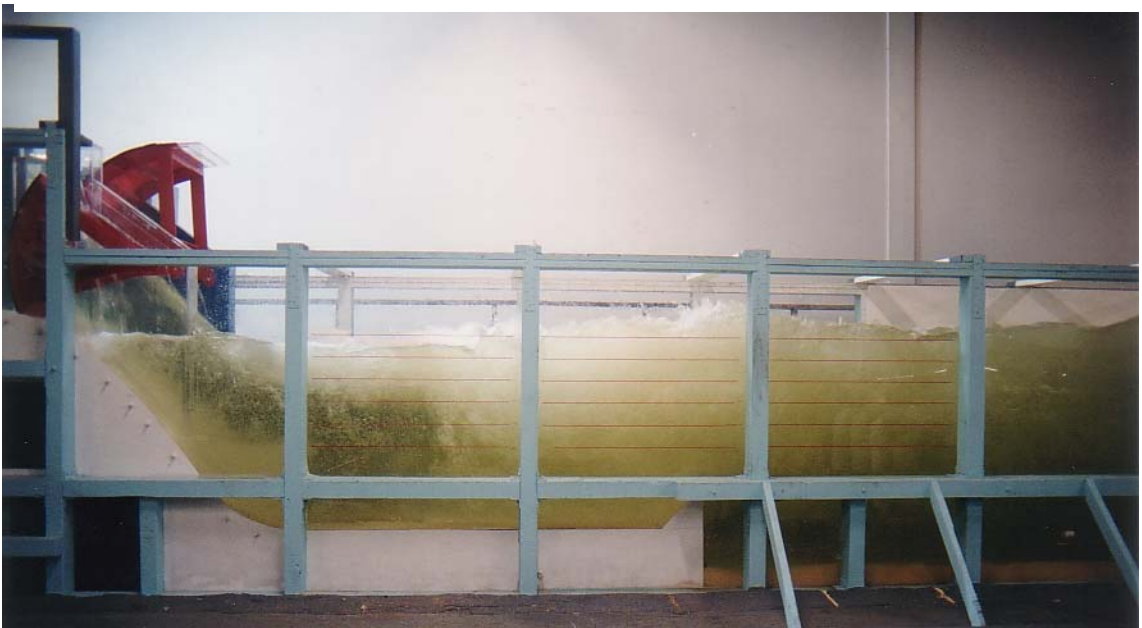
2) Final Design 50 ft Deflector Discharge 112,500 cfs/bay (2,250,000 cfs project discharge) Forebay Water Surface Elevation 276.0 ft Tailwater Elevation 206.0 ft. (R30-14)
