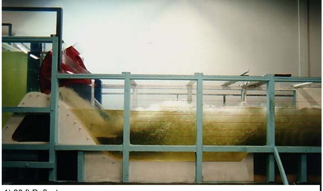
1) 30 ft Deflector Discharge 40,000 cfs/bay (800,000 cfs project discharge) Forebay Water Surface Elevation 268.0 ft Tailwater Elevation 188.5 ft. (R2A-26)
