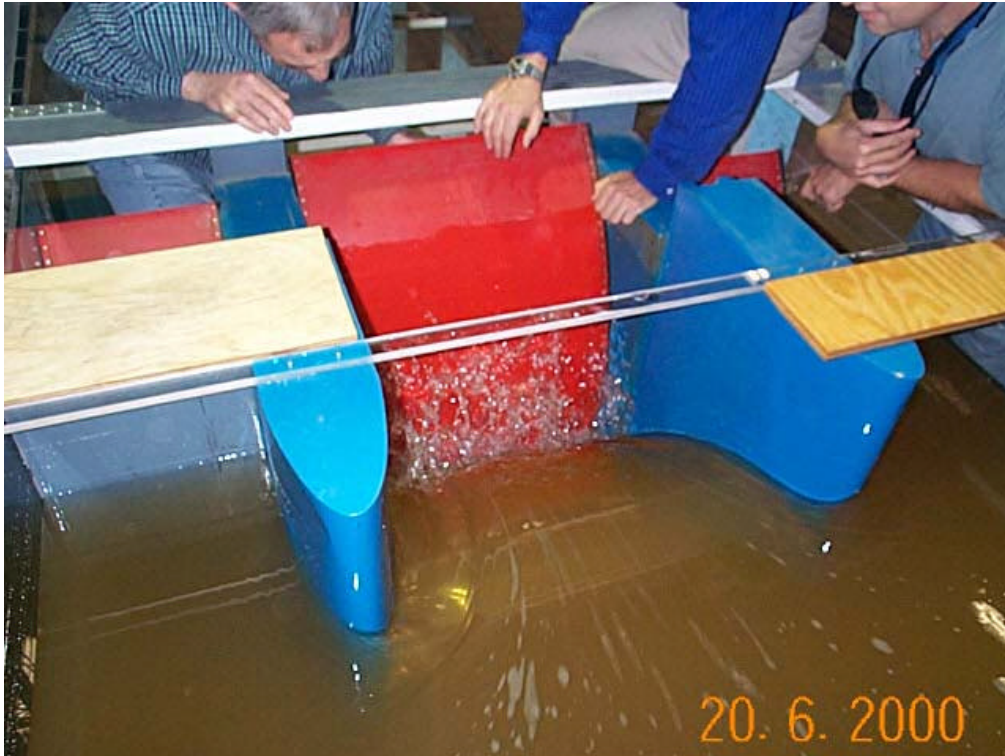
Picture 9. RSW alt 2. Closing tainter gate.
