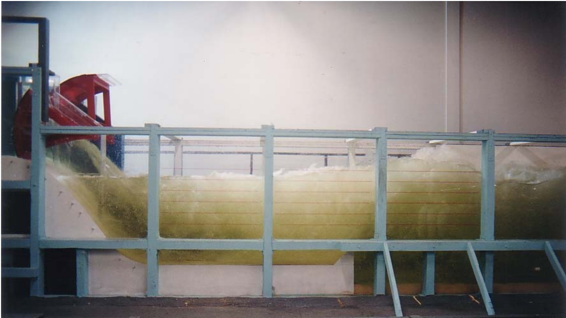
1) Existing Conditions (no deflector) Discharge 112,500 cfs/bay (2,250,000 cfs project discharge) Forebay Water Surface Elevation 276.0 ft Tailwater Elevation 206.0 ft. (R30-02)
