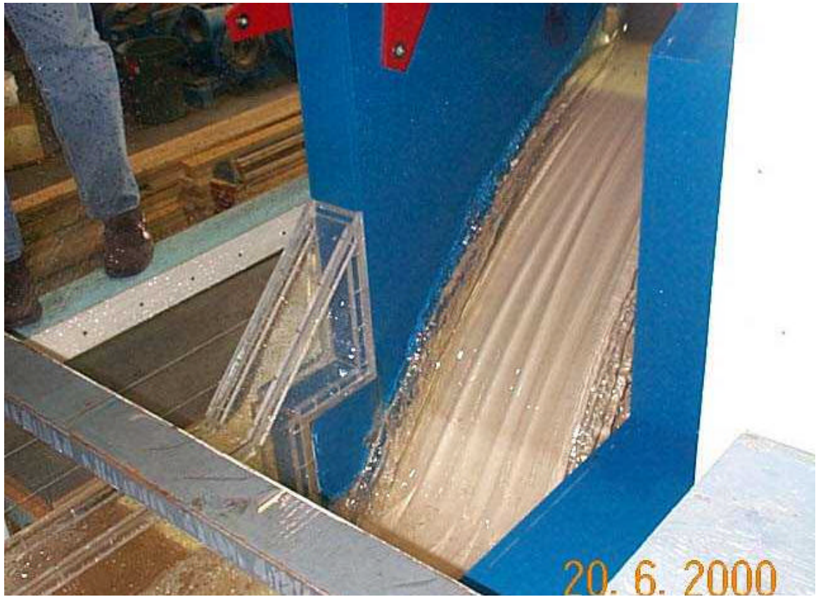
Photograph 3. RSW Alt 2, Roostertails Down Spillway Face
