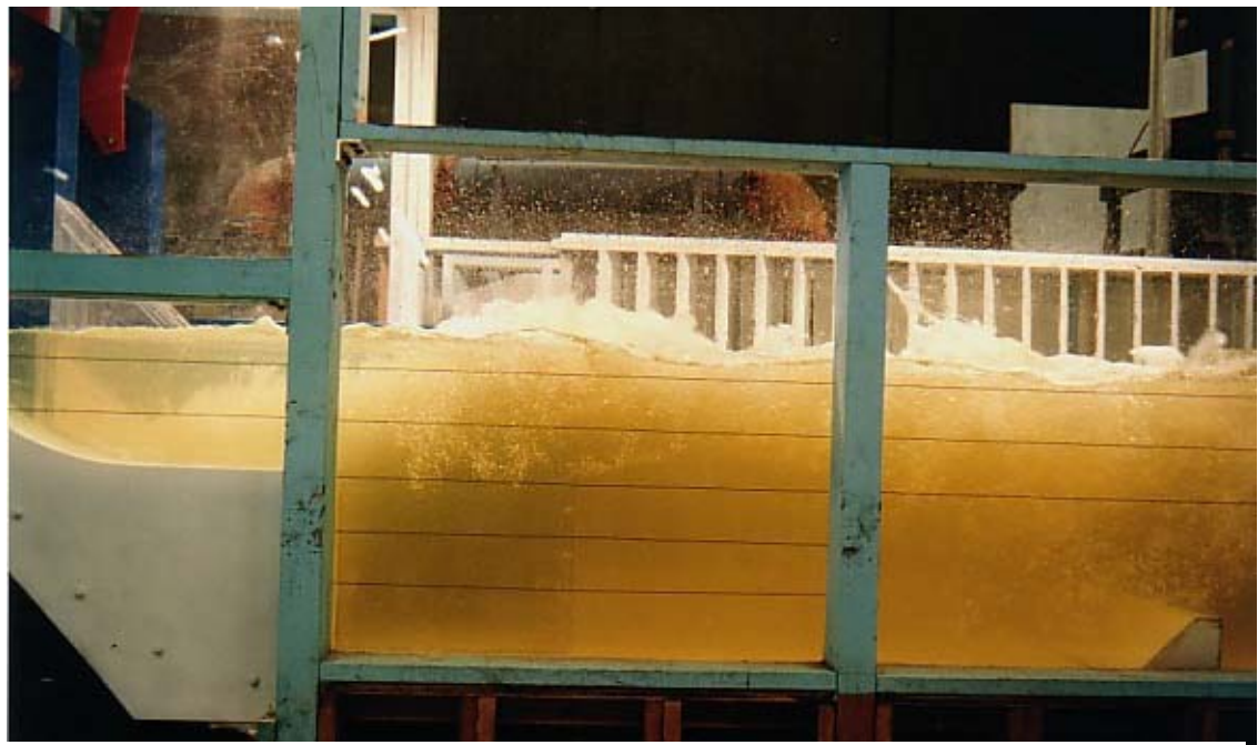
2) Submergence 26.3 ft: Hydraulic jump over the deflector. (R18-31)
