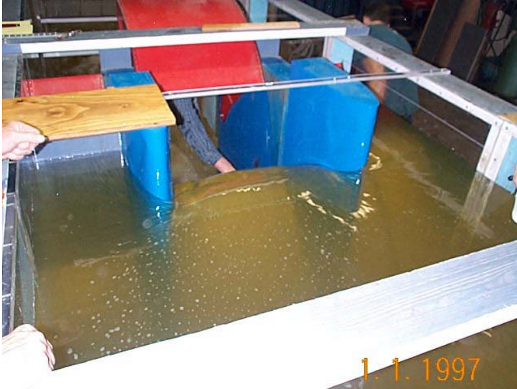
Picture 1. RSW alt 2. Water surface, drawdown around piers.
