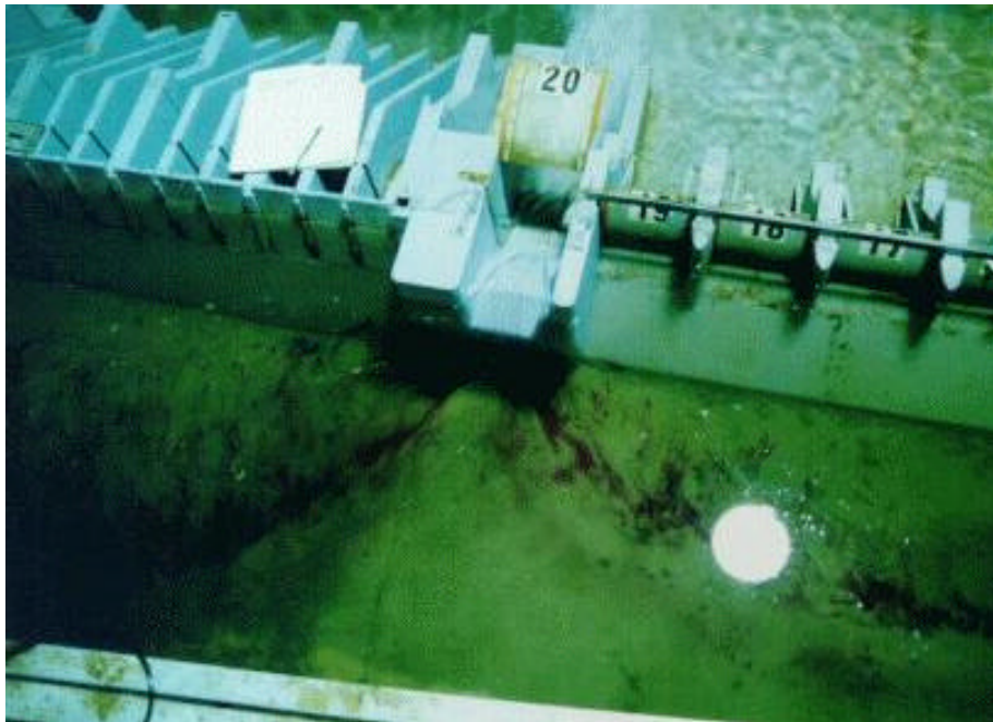
Photograph 17. RSW 7. Approach Flow Conditions, 15.3 kcfs, Total Q 250 kcfs, 30% of Flow Over Spillway (60.8 kcfs)
