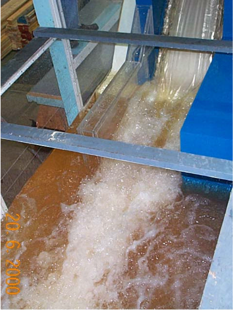
Picture 7. RSW 2. "Rooster tails" and deflector performance.
