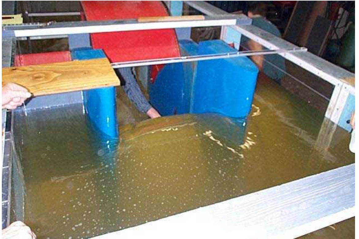
Photograph 1. RSW Alt 2, Water Surface Drawdown Around Piers
