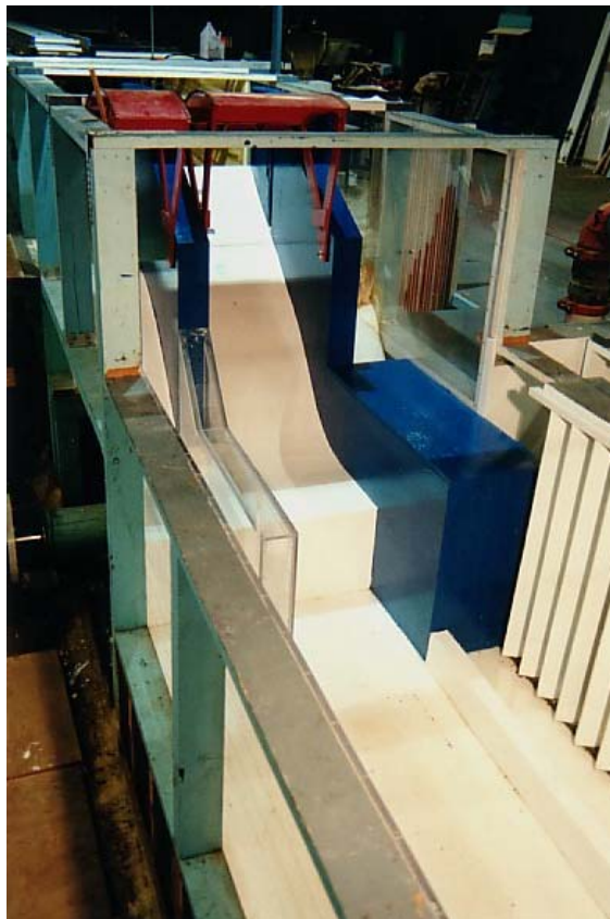
2) Model layout looking upstream toward the Raised Spillway Weir. (R19-07)
